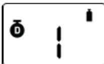
If you set the calibration interval via IR LINK, the remaining day will be displayed. To check the remaining day, press the button until the above image is displayed.
